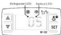
It is a mini-sized and integrated intelligent controller and applicable to the compressor of one Hp.
